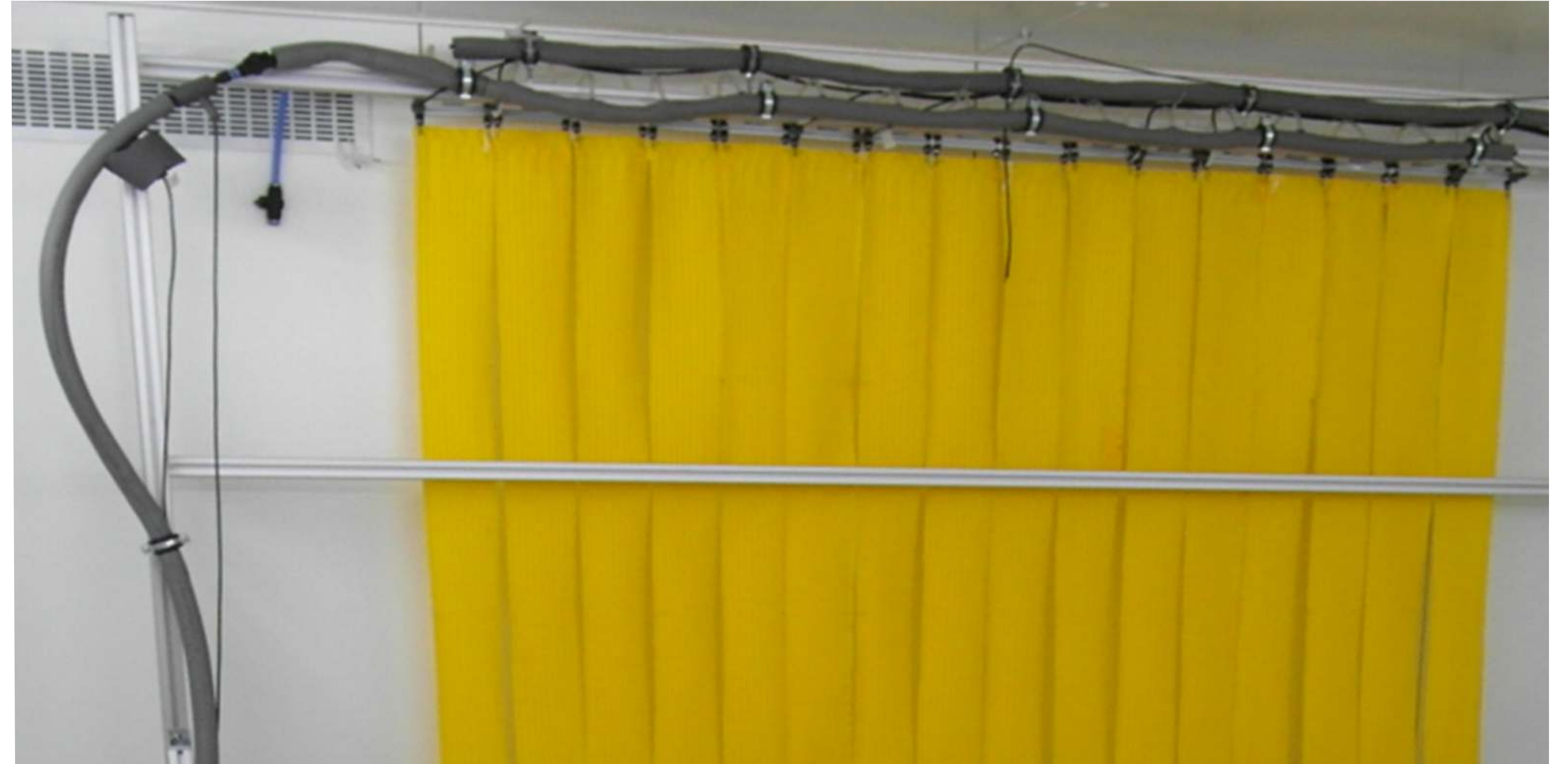
Textile temperature control element (window curtain) as demonstrator (right) and its thermographic image in heating mode
